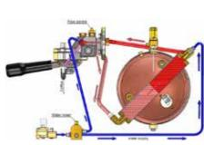
The TCI system in action, showing the hydraulic network and how the coffee water temperature is simply adjusted.
